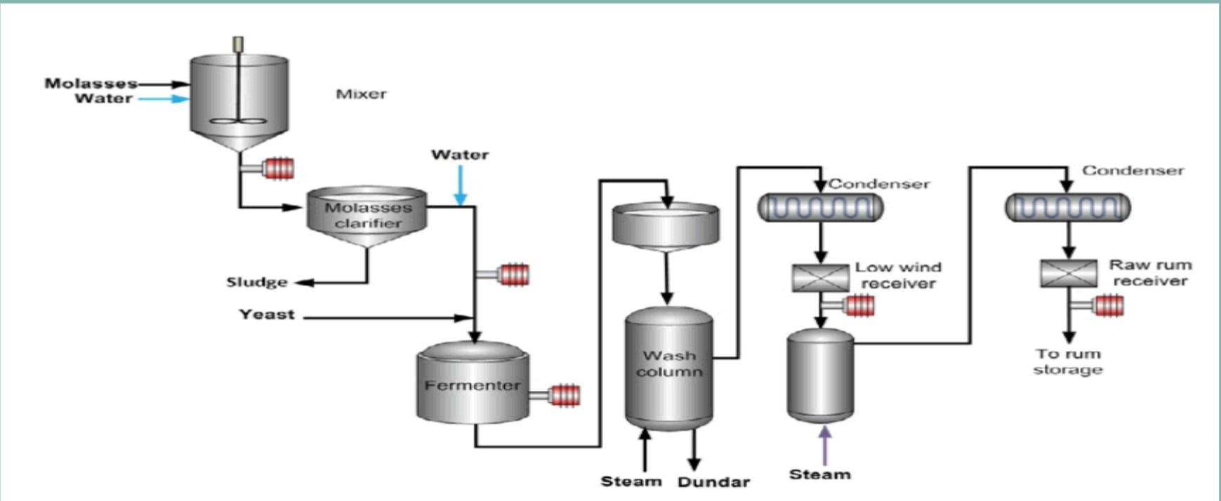
Figure 2: Ethanol production from molasses using fermentation process.
